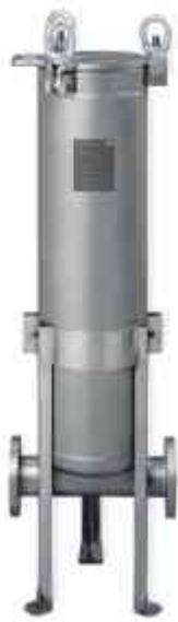
CUNO DuoFLO filter housings are designed and manufactured to economically meet demanding applications. The housings are available for #1 and #2 size DuoFLO filters and are constructed from 304 or 316L stainless steel. DuoFLO housings are designed, fabricated, and "U" stamped in accordance with ASME Section VIII, Division 1 for 150 psi @ 300°F\*. A variety of inlet/outlet connection styles are available (see specification table below).
