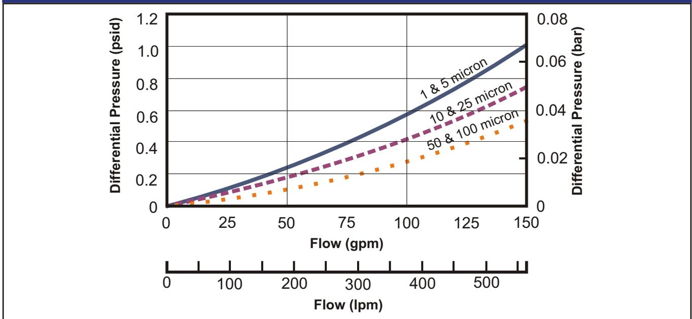
\*#2 Size Element and Support Basket Pressure Drop Only, housing pressure losses are not included.
