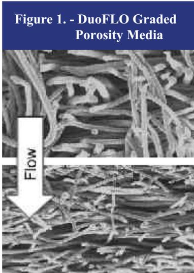
first layer and the finer contaminants in the tighter, downstream layer (Figure 1). The configurations of each nominally rated filter media have been optimized to achieve the longest service life. In addition, media migration is eliminated by thermally bonding the exterior surface of the downstream media layer.
